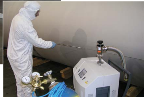
Helium Leak Testing
